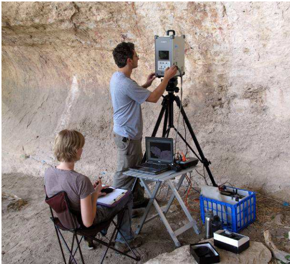
Fig. 11. Triangulation survey conducted at Panther Cave by Geo-Marine, Inc.
