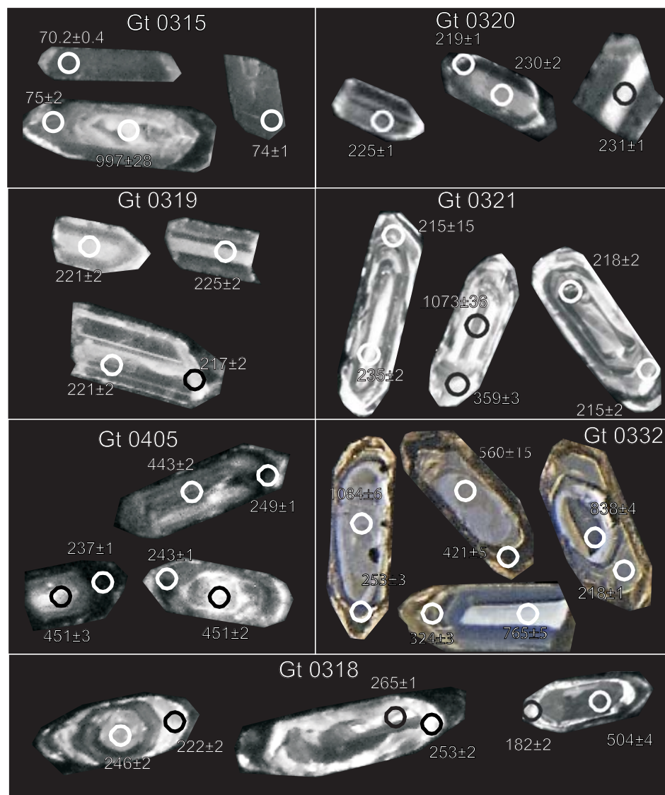
FIGURE 7 | Cathodoluminescence image of some representative zircons analyzed in this work. The circles represent the 34\mu\text{m} LA-ICPMS analyzed spot.
