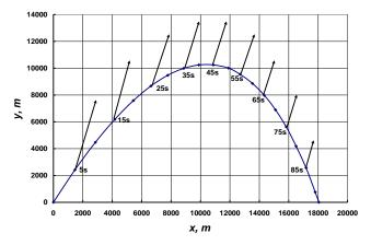
**FIGURE 2.** The jerk vector in projectile motion with launch speed  $v_0 = 600$ m/s; launch angle  $\alpha = 60^\circ$ ; and drag coefficient k = .01/s.
