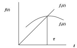
**FIGURE 1.** Graphical solution of Eq. (27). The intersection of  $f_1(t)$  and  $f_2(t)$  furnishes the value of  $\tau$ .
