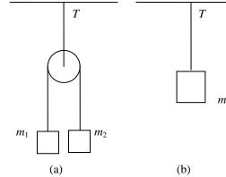
**FIGURE 3.** An Atwood's machine (a) and equivalent system for it (b).
