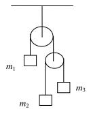
FIGURE 4. An Atwood's machine in series.
