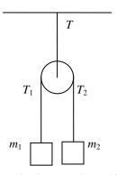
**FIGURE 2.** A simple Atwood's machine, that it consisting of two suspended masses connected by a string that passes over a pulley.
