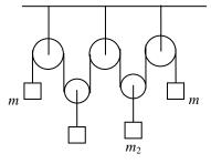
FIGURE 10. the parallel system with two middle masses.
