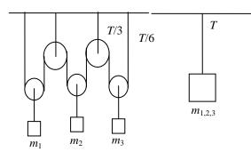
**FIGURE 14.** a) A system including  $m_1$ ,  $m_2$ ,  $m_3$  b) An equivalent system for (a).
