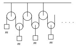
FIGURE 18. An in finite Atwood's machine.
