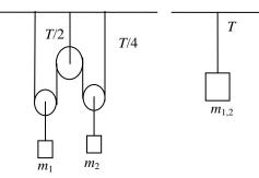
**FIGURE 11.** a) A system including the  $m_1$  and  $m_2$  b) An equivalent system for (a).
