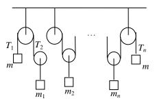
**FIGURE 7.** A parallel network for  $m_1, m_2..., m_n$  and  $T_1=T_2=...=T_n$ .
