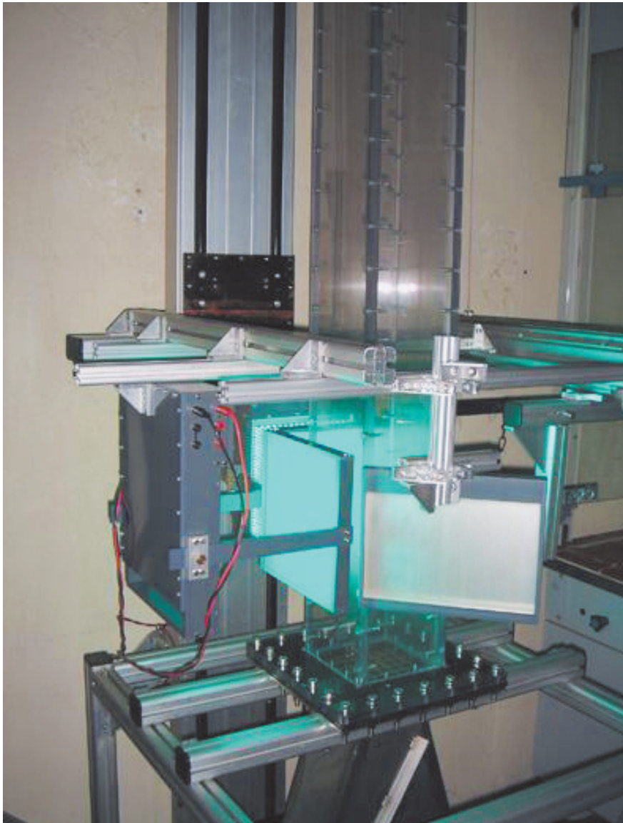
"Stereo PIV arrangement in the bubble column considered in this work."
