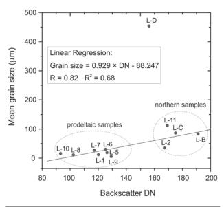
FIGURE 6 | Bivariate plot of backscatter digital number (DN) versus surface sediment mean grain size of HCI-untreated samples. The linear regression ignores surface sample L-D as an outlier. Samples L-A and L-4 are not represented because they lie beyond the backscatter data coverage (see Fig. 5).
