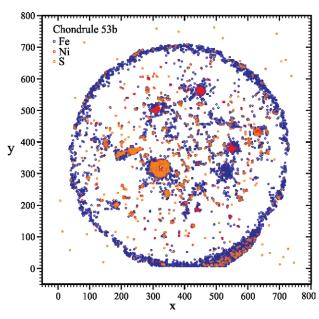
Figure 5. Metal boundaries inside c53b chondrule, determined using an image processing technique, focusing in the nickel, iron and sulphur elements. C53b is an example of iron- and nickel-poor chondrules with iron-rich rims. Observe the nickel and sulphur rich metallic inclusions.
