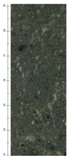
Figure 1. Fragment of the Allende carbonaceous chondritic meteorite (6 cm slab cut from Allende showing distribution of chondrules and refractory inclusions in the fine grained silicate matrix).
